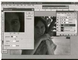
The Unsharp Mask dialog box in Photoshop uses slider controls to adjust Amount, Radius and Threshold.
