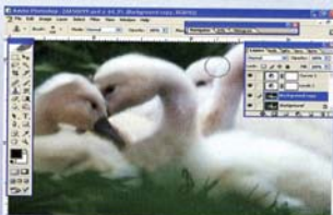
When using Photoshop's Clone Stamp tool, the mouse's pointer on-screen becomes a circle to define your source mark.
